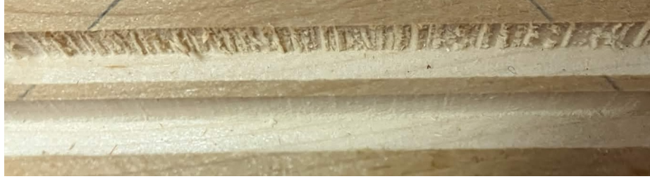
Figure 2.5: A comparison of an optimal (bottom) and non-optimal (top) cutting result.
