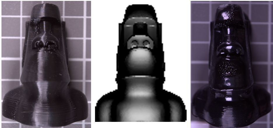
Figure 1: (Left) Original 3D printed Moai statue. (Center) Cubic normal map. (Right) Result polished according to our protocol.
