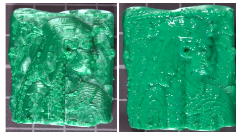
Figure 4: Bas-relief plaque before (left) and after (right) polishing, showing limitations in loss of detail.
